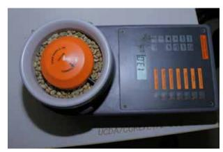
**Figure 77.** A moisture meter for determine moisture level in the coffee
