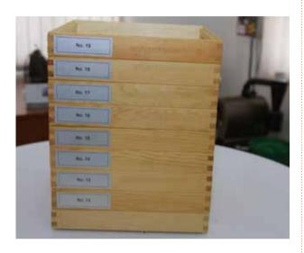
**Figure 76.** Screen size trays for grading green coffee beans
